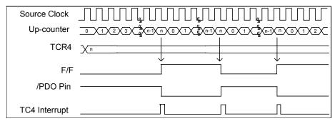
Fig. 5-25 Timing Chart for PDO Mode
